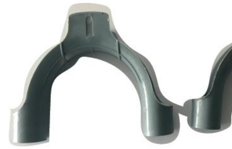
Using these plastic shapes to mould bamboo, once the bamboo has been soaked in warm water so it becomes more flexible and bend
